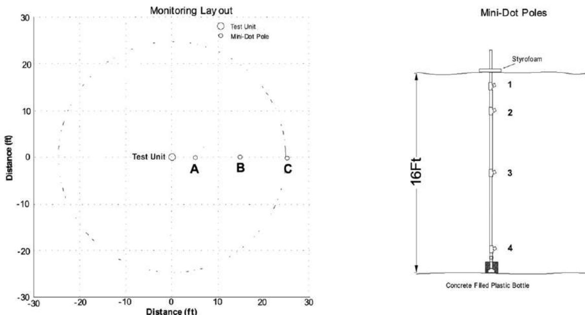
*Field Note on Sensor Positioning: It is noted that due to dynamic environmental factors there is some slight variation from the nominal distances of 3ft, 13ft, and 26ft radii for the fixed-position pole placement*
